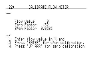
This will set the flow meter to equate 1.5 SCFH to 75% of the maximum of the digital flow meter.
