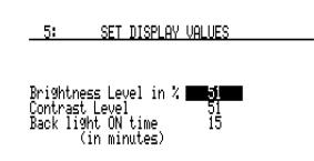
off, the instrument still operates fully, but the display is more difficult to read. To restore the backlight, press any key. To disable this function, enter  $\mathbf{0}$  and the backlight will be always on.
