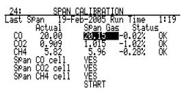
Verify span gas values to Cal Cylinder.
